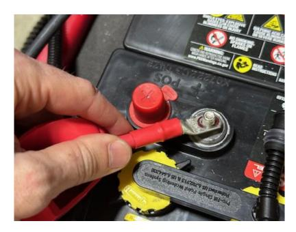
4. Thread the nut that was removed in step 2 back onto the stud.
