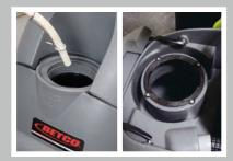
Fill machine with water and cleaning detergent.
