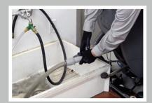
**Empty recovery tank** after each use. Remove hose from housing clip on back of machine, remove cap and let dirty water empty into mop sink.
