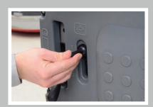
To prevent water from leaking from machine, always raise the solution knob all the way
