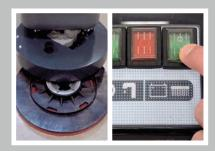
To remove the pad driver (to change or clean pad), power to the machine must be on and the pad driver still raised off the floor. Squeeze the trigger on the handle and quickly release the trigger. This will cause the pad driver to fall to the floor. Then turn off brush switch and vacuum switch.
