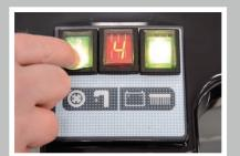
Press to activate brush and suction switch on the machine.
