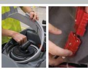
Locate and remove the splash guard from the recovery tank housing. Locate and connect the battery cables.
