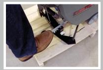
Press and lock pedal on rear right side of machine to lift scrub deck.
