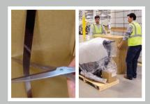
Cut and remove black straps from outside of box. Lift and remove box from top of machine.
