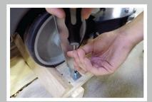
Use Phillip's head screwdriver to loosen and remove metal brackets.
