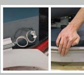
To install splash skirt, engage metal rings with connector nut, and wrap skirt around scrub deck. Lower scrub deck to the floor with your pad/brush installed and slide skirt down to contact the floor.
