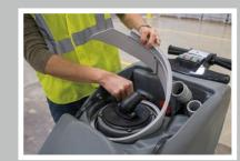
**Brush Skirt and band** clamp, located under recovery tank lid
