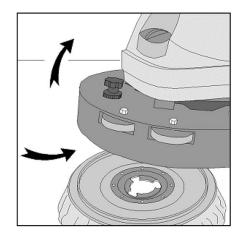
D. Press the operator present control lever (6) and the brush will be hooked automatically.
